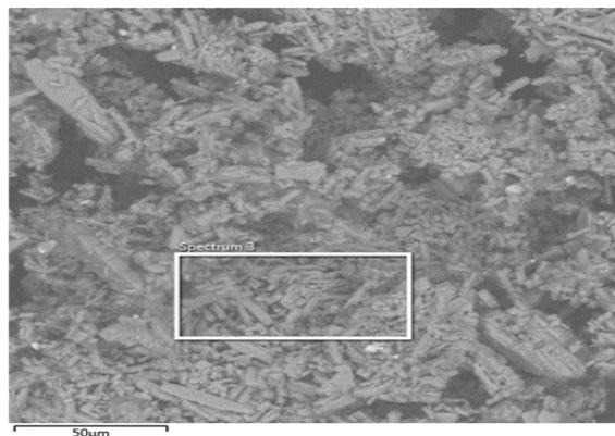
Figure 3: EDS inspection of the phosphogypsum ore
