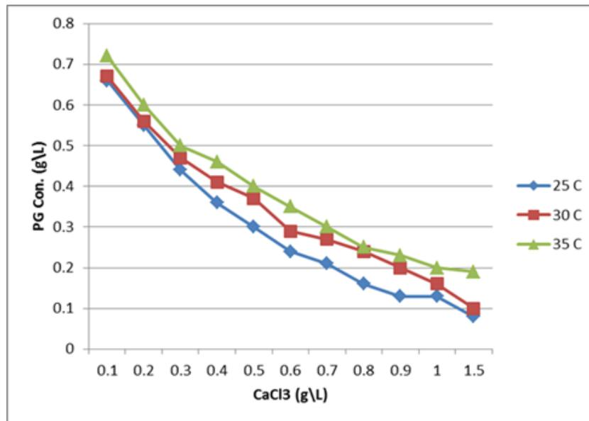
Figure 8: Solubility of phosphogypsum in aqueous solutions of  $\text{CaCl}_2$ .
