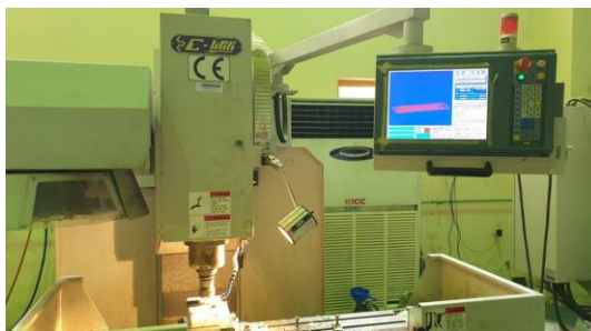
Figure 1: 3-Axis CNC milling machine "C-tek" type
