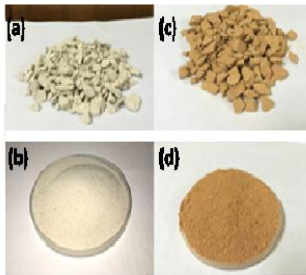
Figure 1: Production of Flint and Kaolin powders from their respective rocks. (a, b) Flint (c, d) Kaolin.
