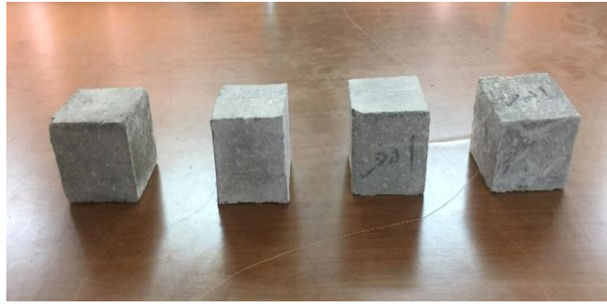
Figure 2: The cement mortars prepared with the incorporation of Flint and Kaolin rocks powders.
