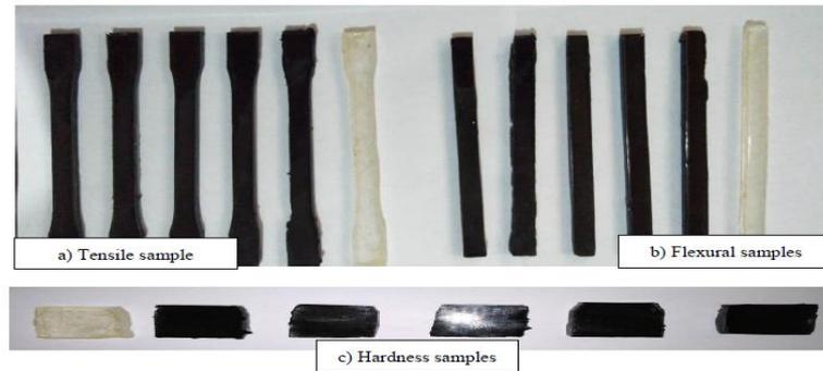
Figure 2: Mechanical test samples
