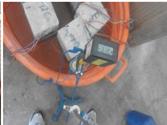
Fig. 5 Half-cell potential test
