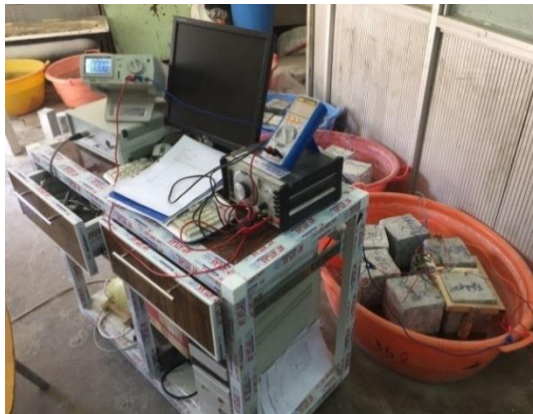
Fig. 3 AC resistance test
