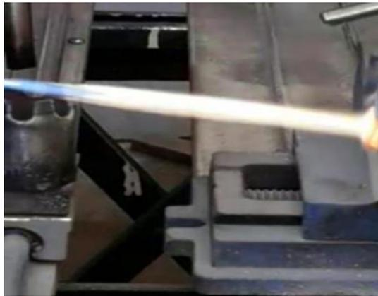
Figure 2: Flame thermal spraying process
