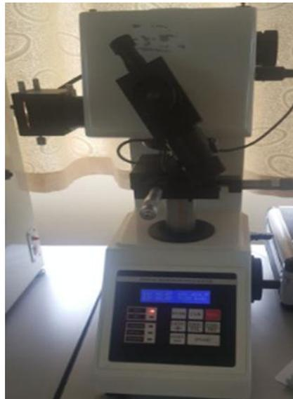
**Figure 3: HVS-1000 Digital Micro hardness Tester.**
