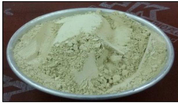
Figure 2: Powder of clay brick waste
