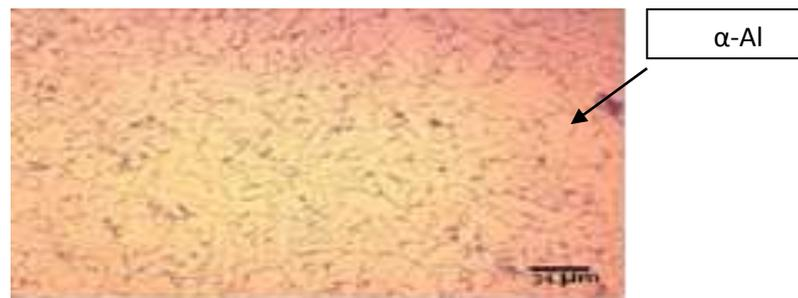
Figure 2: The microstructure of base alloy.
