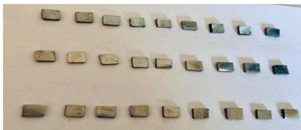
(B) Coated samples after surface machining
