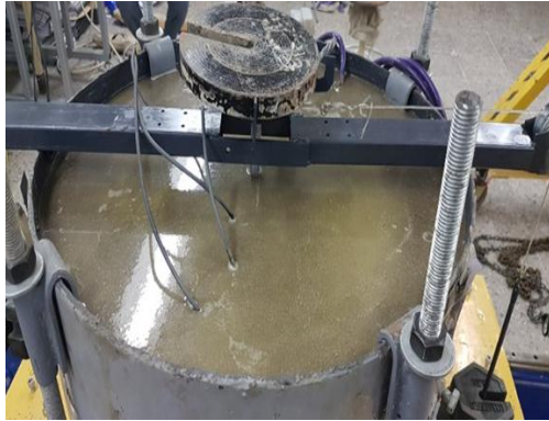
Plate 4: liquefaction phenomena occurred after applying 0.32g acceleration
