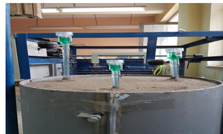
Plate 2: Soil suction test by LT Tensiometer
