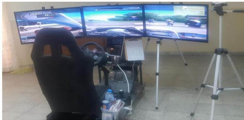
Figure 3: Driving simulator device (Researchers Work)
