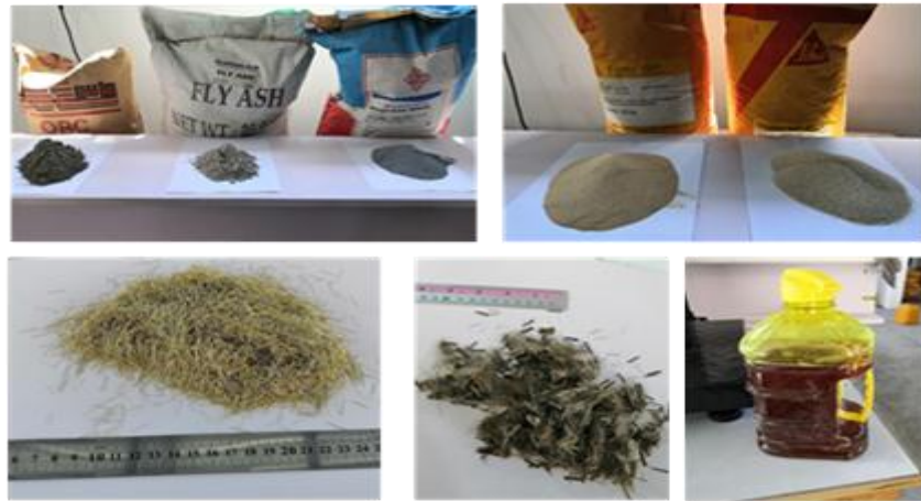
Figure 2: The materials used in experiments; cement, fly ash, silica fume, fine sand, coarse sand, steel fibres, basalt fibres, and HRWRA
