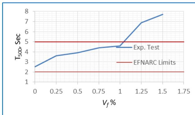
**Figure 2:** Steel volume fraction versus T<sub>500</sub> test
