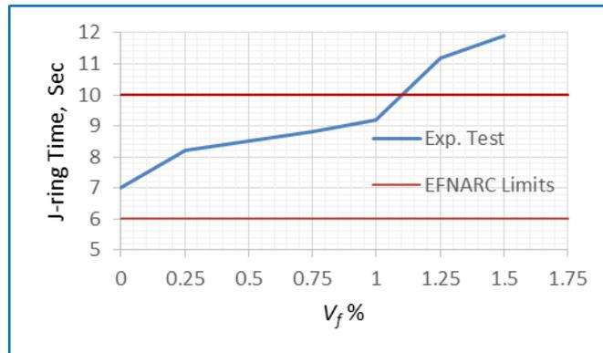
Figure 5: Steel volume fraction versus J-ring test
