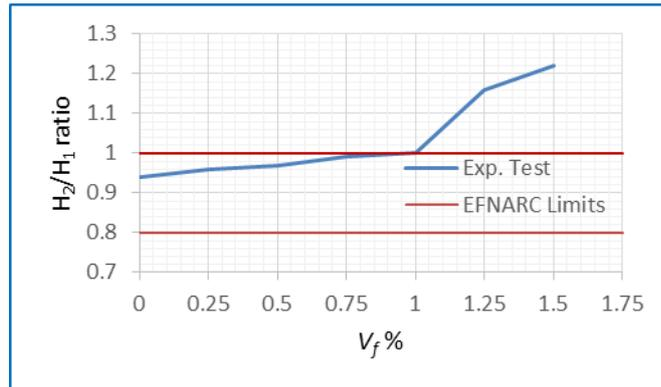
Figure 4: Steel volume fraction versus L-box test
