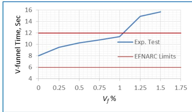
Figure 3: Steel volume fraction versus V-funnel test
