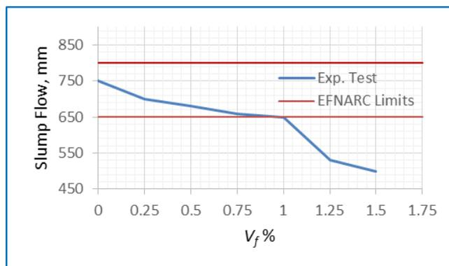
**Figure 1:** Steel volume fraction versus slump-flow test
