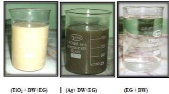
**Figure 5: Shows oxide and metal nanofluid**
