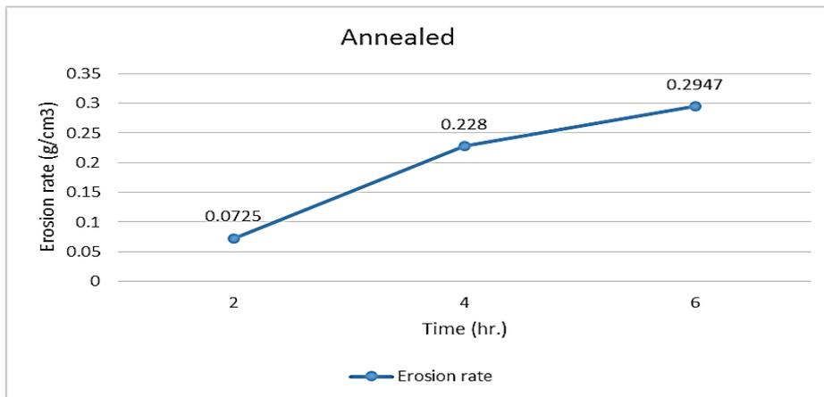
Figure 6: The erosion wear rate of annealed samples at 45° impact angle
