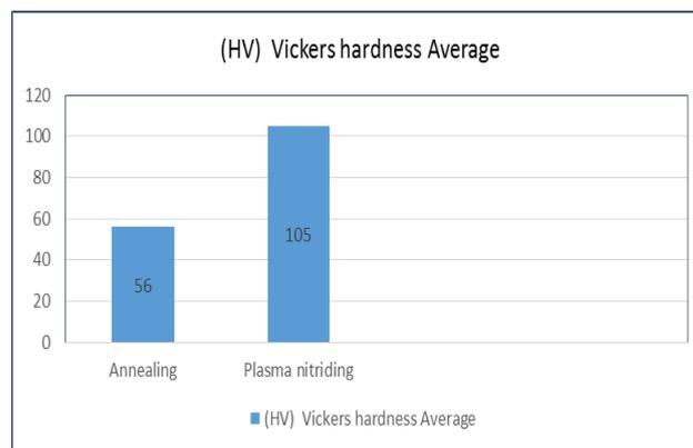
Figure 8: The difference in hardness according to treatment
