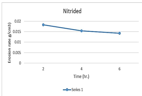
Figure 7: The erosion wear rate of nitrided samples
