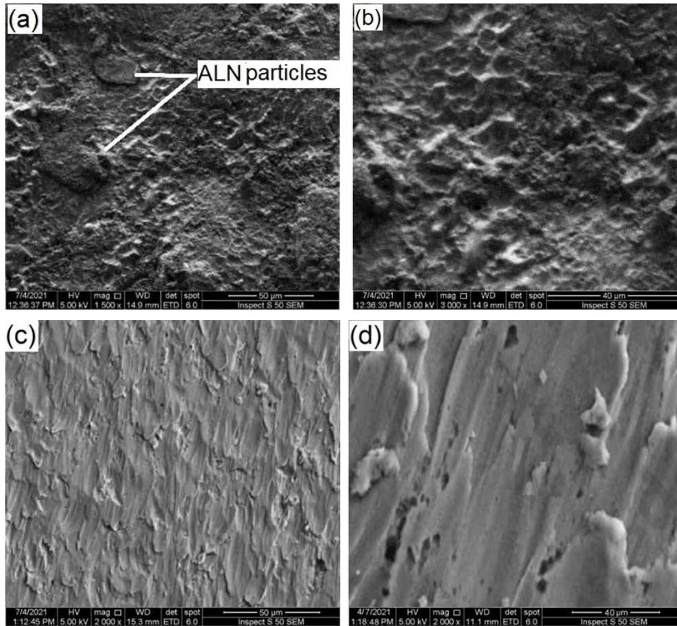
Figure 4: SEM micrographs of the dendritic regions of AlN nitride layer (a)magnification X320 (b) Increased magnification micrograph in (a) X475 (c) eroded nitride samples X360 (d) Increased magnification micrograph in (c) X400
