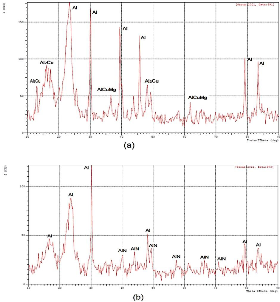
Figure 5: XRD Patterns: (a) Al-Cu 2024 after annealing, (b) After plasma nitriding
